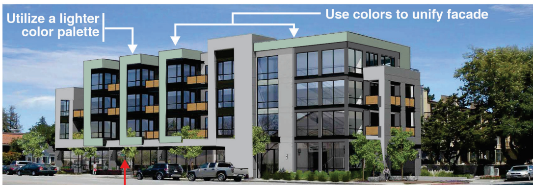
Consider alternate material for ground floor columns (e.g., smooth stone) Recommended Facade Changes
